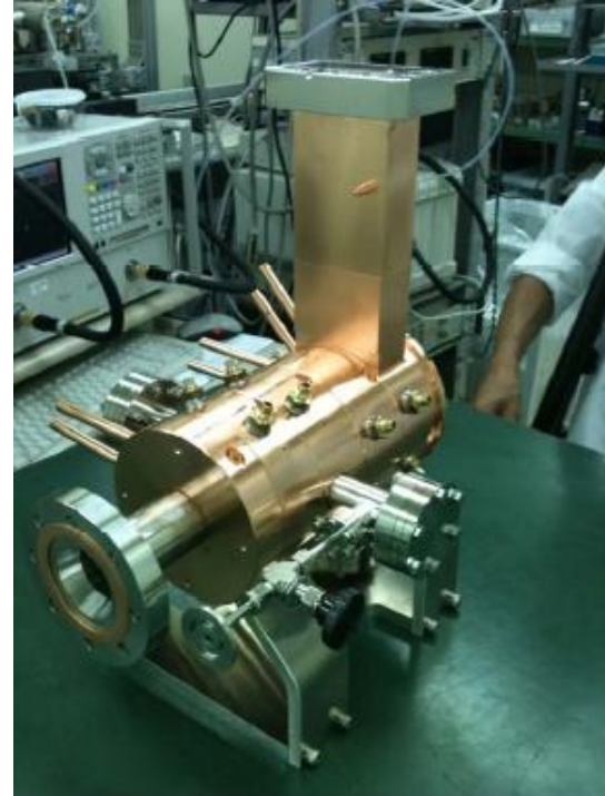
120MV/m, 10MeV S-band Photo-cathode RF Gun
