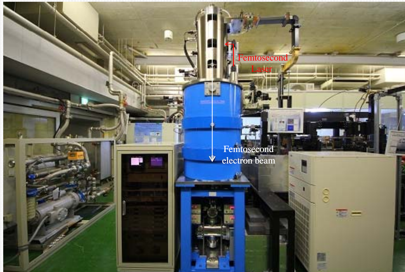
Prototype of MeV UEM (height: 3m, diameter: 0.7m)
