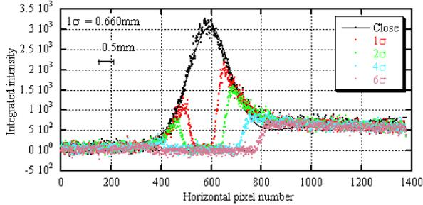
Figure 3: Integrated intensity in horizontal directions of the OTR at the surface of SL1A<sub>ss</sub>. Colored dots indicate the intensities with various scraper gaps. Black dot indicates the intensity under a condition that the scraper fully closed. Black line indicates a result of the gaussian-fit.
