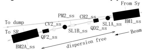
Figure 1: Arrangement of the scrapers in the SSBT line. From the side of upstream, two scrapers were named SL1A<sub>ss</sub> and SL1B<sub>ss</sub>. Blocks indicate the magnets.
