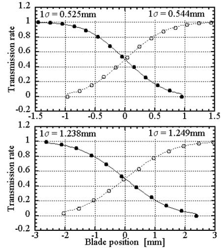
Figure 4: Upper and lower figure show the transmission rate versus blade position at SL1A<sub>ss</sub> and at SL1B<sub>ss</sub>, respectively. Closed and open circles indicate the rate for left- and right-blade, respectively. Solid and broken lines indicate the results of a least-squares fit with an error function.
