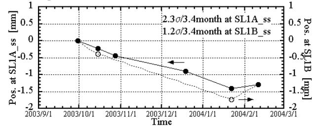
Figure 7: Long-term change in the position of the effective beam center at the scrapers. Closed and open circles indicate the changes at SL1A<sub>ss</sub> and at SL1B<sub>ss</sub>, respectively.
