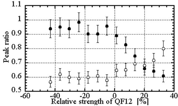
Figure 5: Peak ratio, which was defined as a ratio of the intensity at the horizontal center of the collimated beam to that of no-collimated beam, versus relative strength of QF12<sub>ss</sub>. Black circle and dot indicate the ratio for SL1A<sub>ss</sub> and that for SL1B<sub>ss</sub>, respectively. Error bar indicates one standard deviation of the intensity fluctuation of the ejected beam from the booster.
