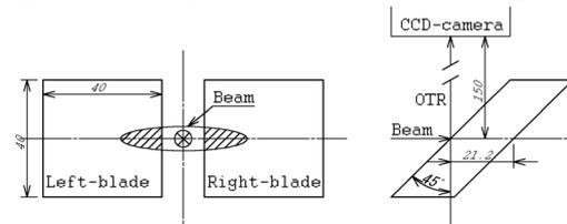
Figure 2: Detail of the scraper. Left- and right-side figures show an elevation view and a cross-section view, respectively.
