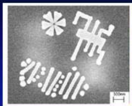
SEM image of Ni pattern on SiN
