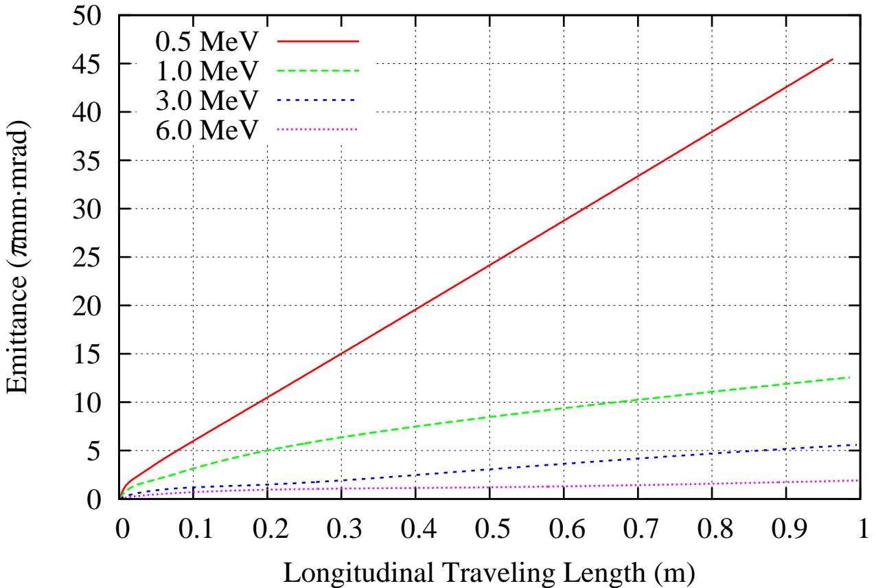
Pulse width: 200 mm,  $\epsilon = \langle \gamma \rangle \langle \beta \rangle \sqrt{\langle x^2 \rangle \langle x'^2 \rangle - \langle x \cdot x' \rangle^2}$
