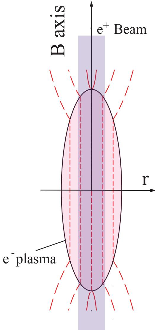
$$V(r) = (n_e e r^2) / (4\epsilon_0) \\ = \beta n_e (\text{cm}^{-3}) r^2 (\text{cm}) \\ (\beta = \sim 4 \times 10^{-7} \text{ V cm})$$
