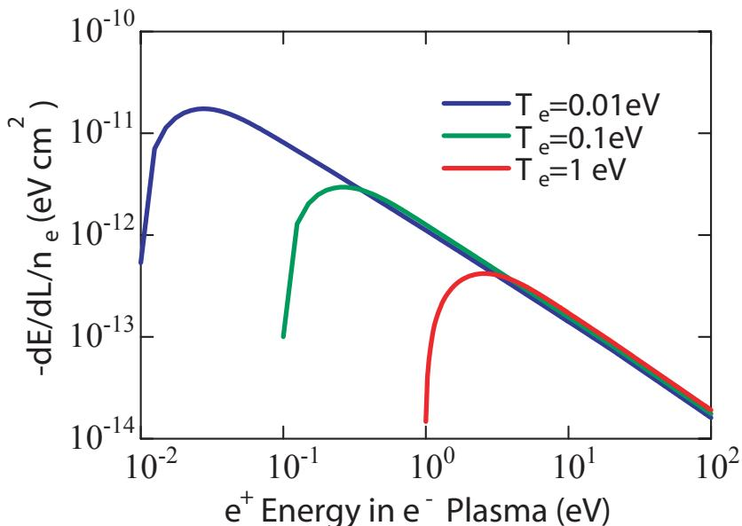
$$-dE/dL(\text{eV/cm}) = \alpha n_e(\text{cm}^{-3}) / E(\text{eV}) \quad (\alpha \approx 1.5 \times 10^{-12}, \text{ if } T_e < E)$$
