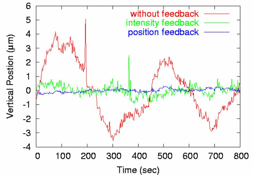
RMS:  $1.98 \mu\text{m}$ ,  $0.37 \mu\text{m}$ ,  $0.13 \mu\text{m}$
