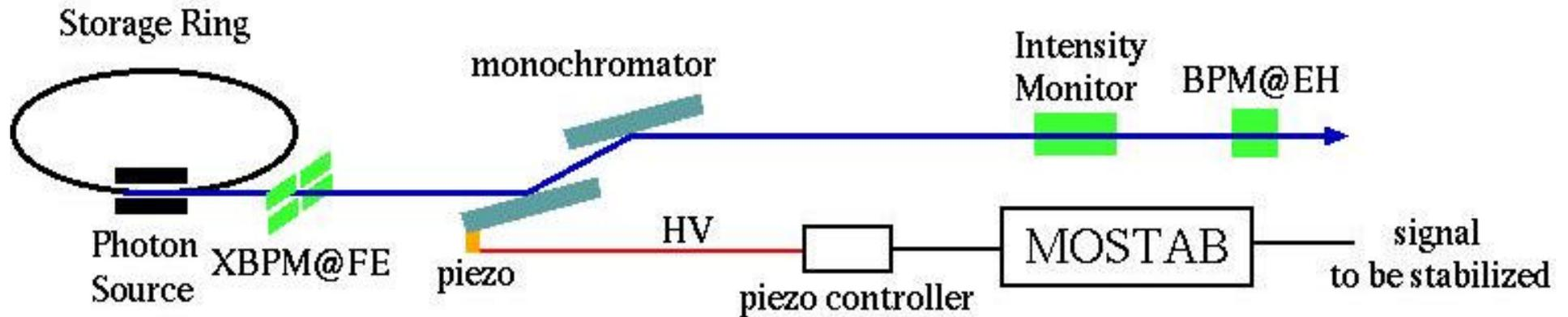
**MOSTAB (Monochromator Stabilization)** module applies a feedback voltage to the piezo actuator of DCM.
