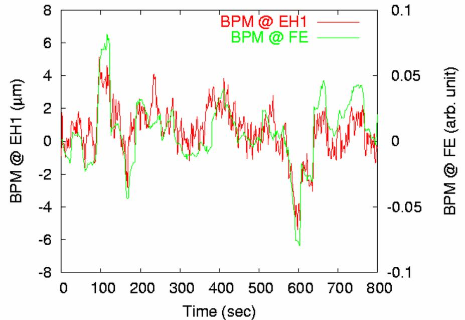
Simultaneous stabilization of x-ray beam intensity and position was not possible due to electron beam instability.
