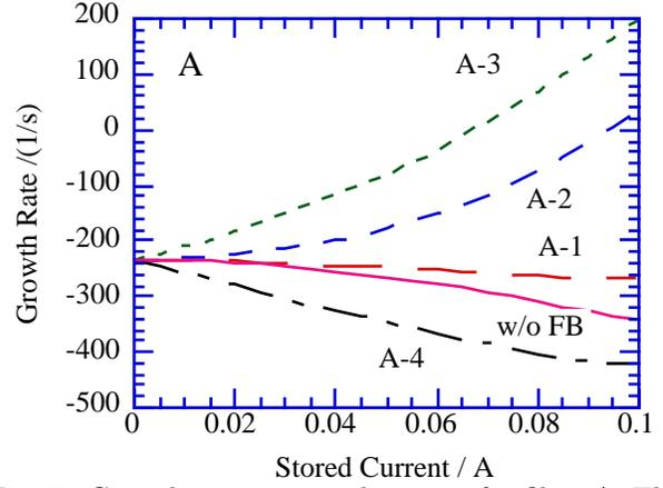
Fig. 5 Growth rate vs stored current for filter A. The growth rate includes radiation damping.
