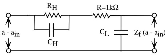
Fig. 2 The filter circuit  $Z_f$  in a feed-back controller of the SPring-8 storage ring. The values of  $R_H$ ,  $C_H$  and  $C_L$  are listed in Table 2.
