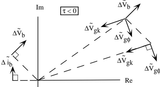
Fig. 7 Phasor diagram of the small shift of the cavity voltage.  $\tilde{V}_b$  is produced by small timing delay of the beam for  $\tau < 0$ .  $\tilde{V}_{gk}$  and  $\tilde{V}_{g\phi}$  are voltage produced by the amplitude and the phase feed-back loop to  $\tilde{V}_b$ . The static part of voltages are the same as Fig. 1.
