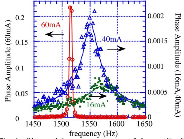
Fig. 8 Observed frequency response of the amplitude of phase oscillation of the beam with Filter B. The data for 60mA is 2 magnitude larger than the data at 16mA and 40mA. The damping time/rate of the synchrotron motion from the width of the data are  $5.5ms/182s^{-1}$  for 16mA,  $12ms/83s^{-1}$  for 40mA and are the expected value from the theory, shown in Fig. 6. the beam was unstable at 60mA. The peak height is also proportional to the damping time.
