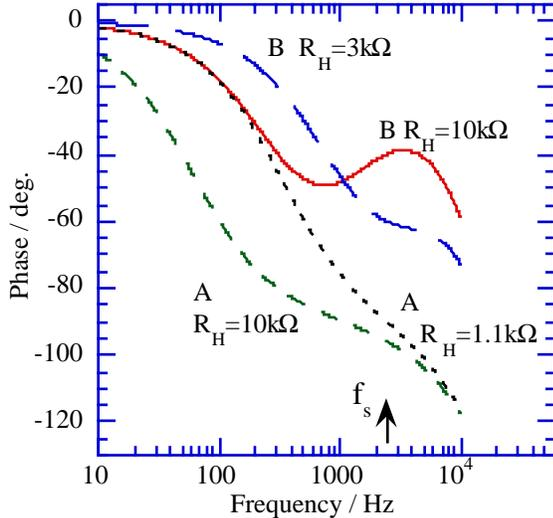
Fig. 3 Phase shift of the feed-back loop without beam current for parameters listed in Table 2.
