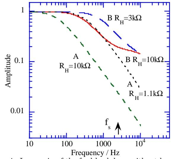
Fig. 4 Loop gain of the feed-back loop without beam current for the parameters listed in Table 2
